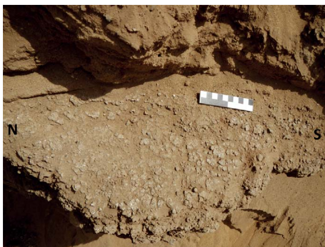
Fig. 91 Exposed horizontal surface of the clay bed with desiccation cracks (photo J. Trzciński)
